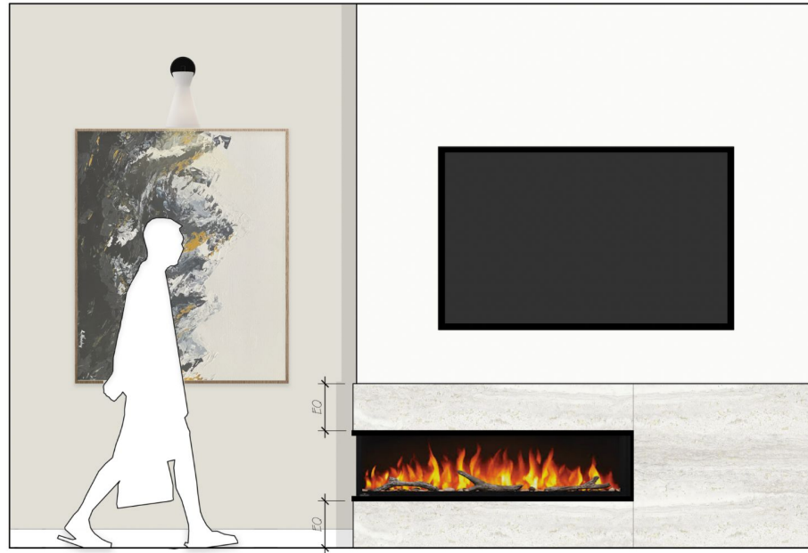
Sketch: Fireplace Wall, Front Reference for Material Placement & Millwork Layout Verify all design details/dimensions on-site and with final Fireplace Specifications
