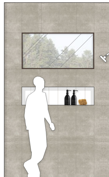
Sketch: Shower Wall Reference for Material Placement only Niche Size TBD - verify on-site with tile layout
