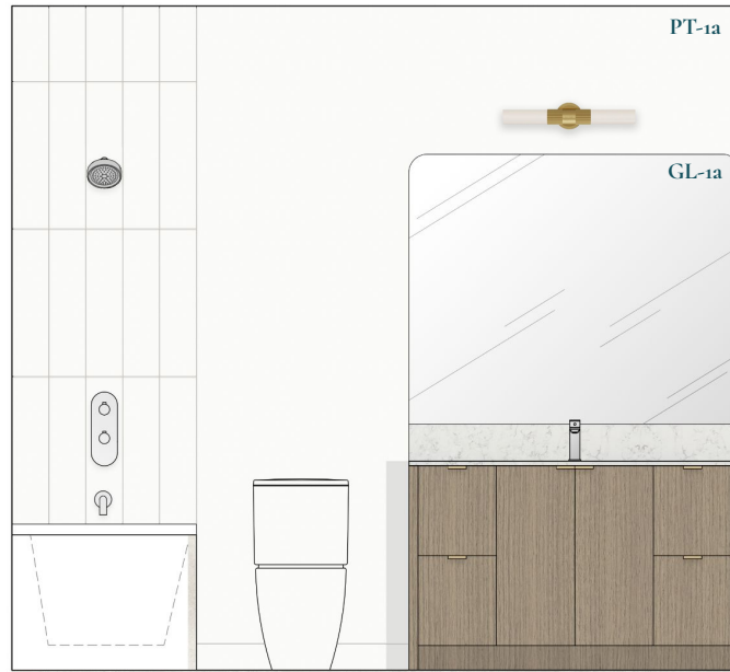
Sketch: Vanity Wall Reference for Material Placement & Millwork Layout Does not depict actual Plumbing Fixtures
